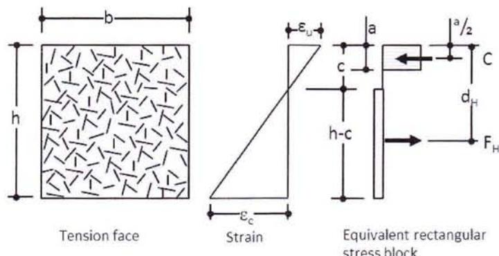
**Figure 2 – Helix Force Equilibrium and Strain Compatibility Diagram**
